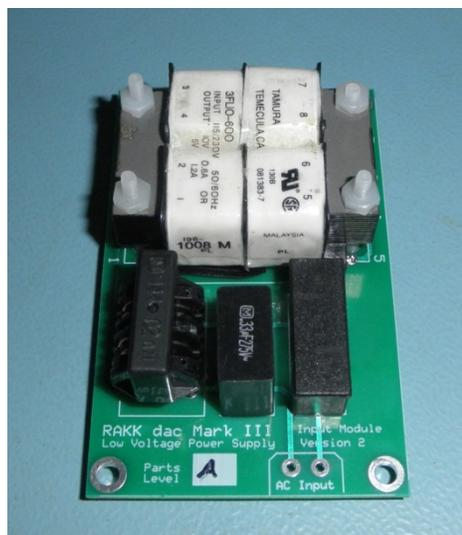
The Input Module takes the mains line voltage (120VAC or 230VAC) and produces an output of 6VAC. This module is capable of providing power for a single Output Module. While the output voltage is nominally 6VAC, the actual voltage will vary depending on the amount of current drawn by the load.
