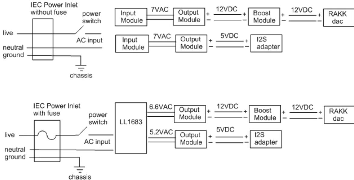
The above figure shows two different low voltage power systems.
