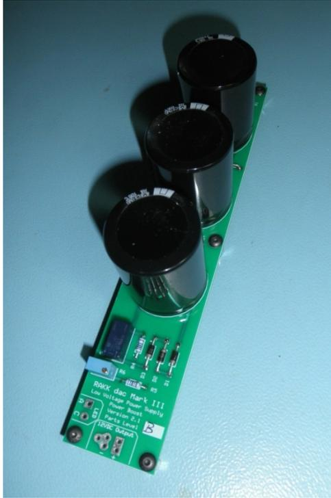
The Power Boost Module is inserted between an Output Module and a RAKK dac, providing additional capacitance needed by the RAKK dac for optimal performance. An I2S adapter does not use a Power Boost Module.
